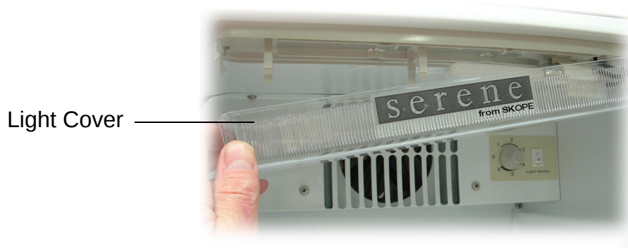
Figure 5: Removing the Light Cover
